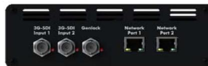
End view showing BNC for Electrical I/O
