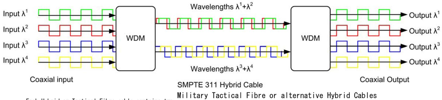
Each Hybrid or Tactical Fibre cable contains two singlemode fibres.
